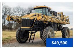
2012 AGCO Rogator 1100, 5049 hours, AGCO Power T4 8.4L 370 hp diesel engine, 1100 gal. SS tank, 100 ft booms with SS boom lines, 10 in. nozzle spacing, 5-way nozzles body, 7-section shutoff valve, Raven Viper Pro, AutoSteer, AccuBoom, A/C, AM/FM radio, air ride seat, 380/90R46 tires (30% remains).
