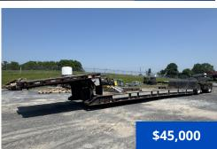
2014 BWS EZ 2 Load Trailer, Overall length of 53 ft, and 102 in. wide low boy trailer, 18,881lb empty weight 30' deck, trailer air operated, 1 ½ inch softwood floor on the gooseneck, and a mix of 1 ½ inch softwood and hardwood on the lower deck, with 3/16 inch formed deck plate over the wheels, Two or three axles of 25,000 lb capacity each, Ridewell RAR 240 U/S suspension, 6 ½ inch air ride 25,000 lb - includes air gauge and dump valve enclosure, 255/70R22.5 tires.
