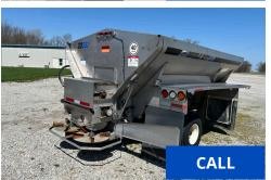
**2021 GVM Double Duty SS1,** 11 ton, 13 ft x 102 in. wide, 330 ft<sup>3</sup> capacity, 304 SS cross member and mounts, peaked end plates, PWM valves with RCM ISO spinner and drag controls, Heavy Bulk Standard Rotation spinners, 34 in. #3 conveyor chain with wiper, rate sensor, bulkhead window, 304 SS frame cover, 124 in. float fenders, and rear camera.
