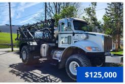
2016 Peterbilt Stahly PB348, 1679 hours, 11,429 miles, Peteriblt chassis, PX-9 350 hp diesel engine, automatic trans., 1450 gal. SS tank, 80 ft booms with SS boom lines, 20 in. nozzle spacing, 5-section shutoff valve, 5-body nozzles, Raven Viper 4 controller, foam marker, AM/FM, A/C, air ride seat, fenders, front 48x25.00-20 Michelin (80% remains) rear 66x43.00-25 Alliance tires (70% remains). Includes set of row crop tires (90% remains). Excellent Condition!
