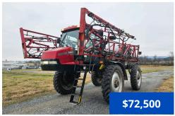
**2013 Case IH Patriot 3330**, 4025 hrs., Fiat 6.7L 285 hp diesel engine, hydrostatic trans., 1000 gal. SS tank, 90 ft. booms with 20 in. nozzle spacing, single body nozzles, SS chemical eductor, Trimble FMX2000 controller, AutoSteer, Auto shut-offs, AIM Command nozzle control, A/C, AM/FM radio, air ride seat, fenders, 380/90R46 Firestone tires (70% remains).
