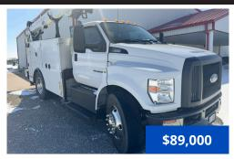
2017 Ford F750 Super Duty, 201,185 miles, 6.7L power stroke diesel engine, automatic transmission with PTO provision, 50 gal fuel tank, air brakes, extended cab, 11ft. utility body, 8 drawer tool box, adjustable shelves, power distribution box with hose/ reel, 10,000 lb lifting capacity crane, 100 PSI air compressor, back-up alarm, 158 in wheelbase, 22.5 front/rear wheels.
