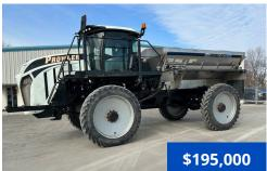
2019 GVM T380 Prowler, 2680 hrs., Cummins QSL9 380 hp turbo diesel engine, Funk DF250 4x4 powershift 11-speed auto. trans., Dromos fixed axles, 2WS, sprayer combo joystick, reverse pitch fan, 304SS GVM 11.0T Double Duty spreader body, bulkhead window, Raven Viper 4 with RS-1 ISO steering receiver, A/C, AM/FM/BT radio, air ride seat, electric roll tarp, front and rear fenders, 380/90R46 Goodyear tires (60% remains).
